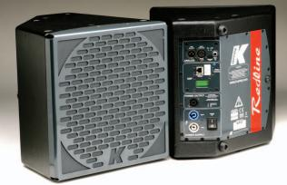
The KF12 uses a 12" neodymium speaker with a 3" voice coil for low-mid frequencies. The mid-high frequency section uses a co-axially mounted 3" voice coil neodymium compression driver
